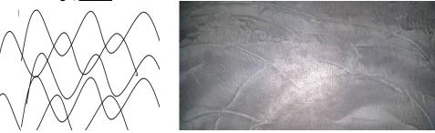
Distribute the Quartzline Cementitious Micro BASE with a curved wave motion. Using the same motion apply the Cementitious Micro TOP.
