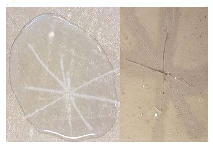
Photo on the left above shows that water is unable to get underneath the lacquer whereas on the right water has clearly been absorbed.
